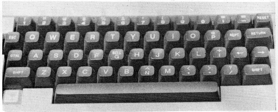
Fake Apple keyboard. Note how the metal tray at the bottom protrudes from the body of the machine.
