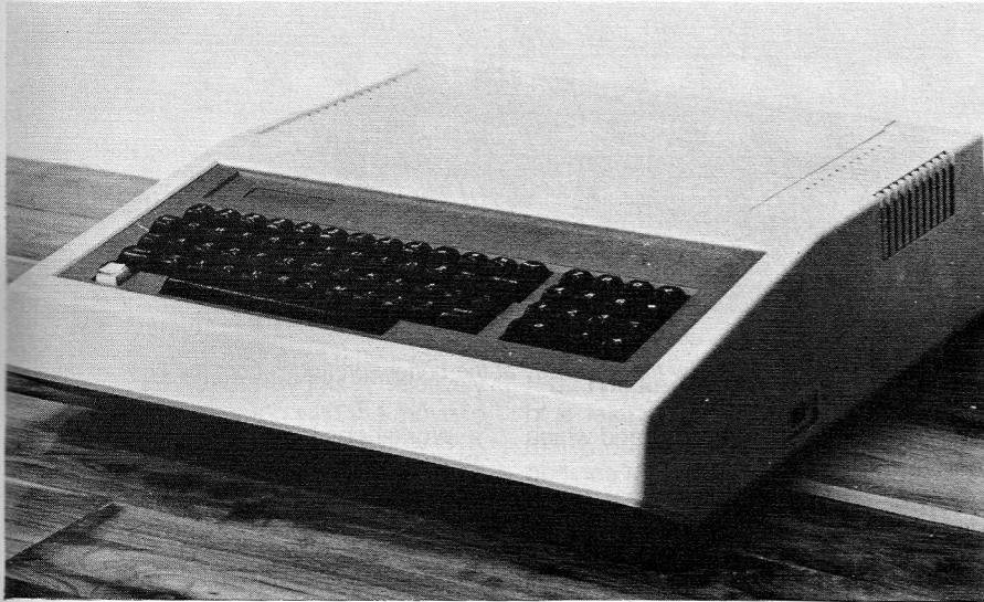
One of the newer fake Apples, with a numeric keypad and different case. This machine is comparatively reliable.
